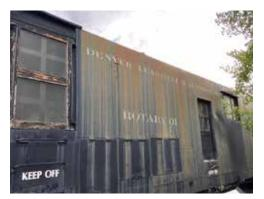
The rotary snowplow received a fresh coat of paint, after suffering from years of deterioration. Lead paint abatement required contractors to construct a sealed "tent" around the rotary snowplow before work could begin. Painters will apply the final stenciling spring 2022.
